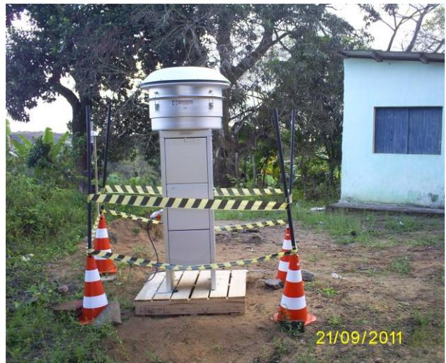
(b) AGV MP<sub>10</sub> ECOTECH-HVS 3000.
