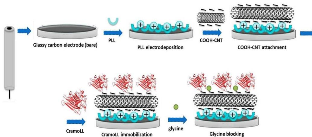
Scheme 1. Schematic representation of sensor construction steps.
