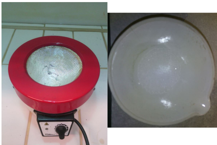
Figure 5.1: Hot blanket used in the synthesis and ceramic capsule with urea
