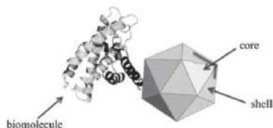
Figure 3. Schematic representation of a core-shell quantum dot functionalized and conjugated with a biomolecule.
