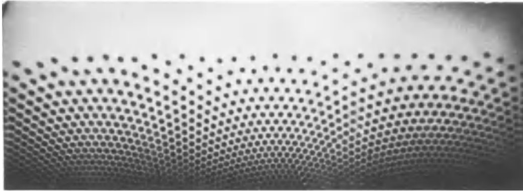
Figure 1.3 Configuration of magnetized steel balls in a tilted box. The "gravity rainbow" pattern (from [15]).
