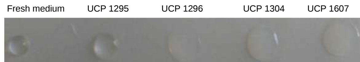
Figure 2: Tensoactivity of crude biosurfactants of the Rhizopus strains on parafilm M hydrophobic surface.
