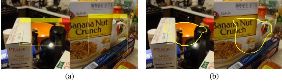
Figure 4.3: Examples of detection represented with (a) bounding box and (b) recognized object contour.
