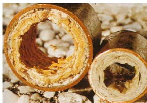
Fig. 1 Scale removed from a water pipe sectioned from a boiler
