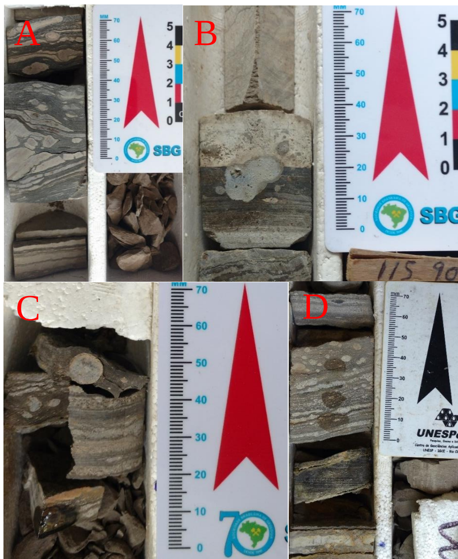
Figura 20 - Exemplos da Fácies Carbonato pelóidal (Cp). Legenda: A – PS04CE ~ 102,00m; B – PS07CE ~ 118,00m; C – PS13CE ~ 145,00m; D – PS10CE ~ 99,00m.
