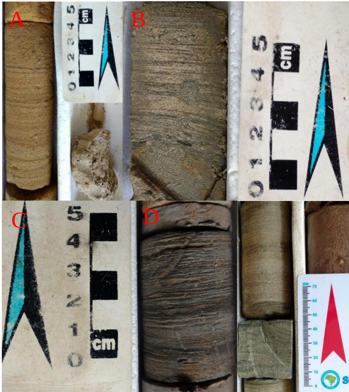
Figura 12 - Exemplo da Fácies Arenito laminado (Al). Legenda: A – PS02CE ~ 35,00m; B – PS10CE ~ 34,00m; C – PS08CE ~ 47,00m; D – PS07CE ~ 62,00m.
