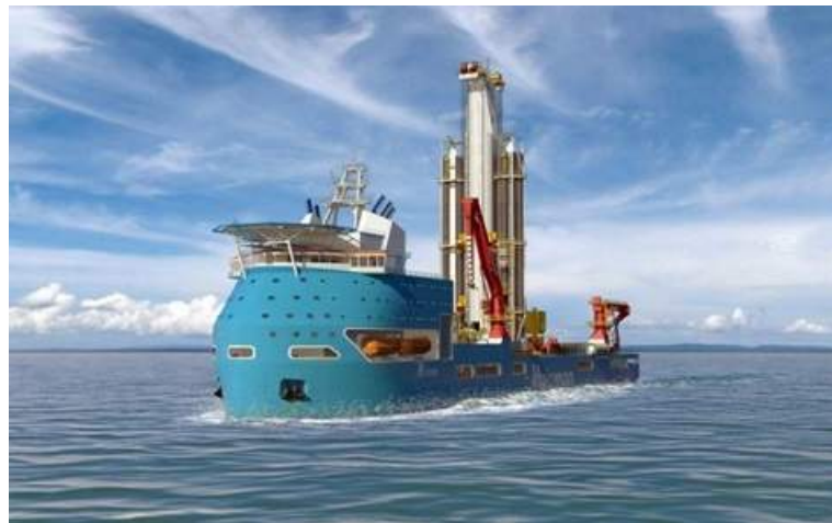
Figure 1: Example of drill ship: Huisdrill 12000.
