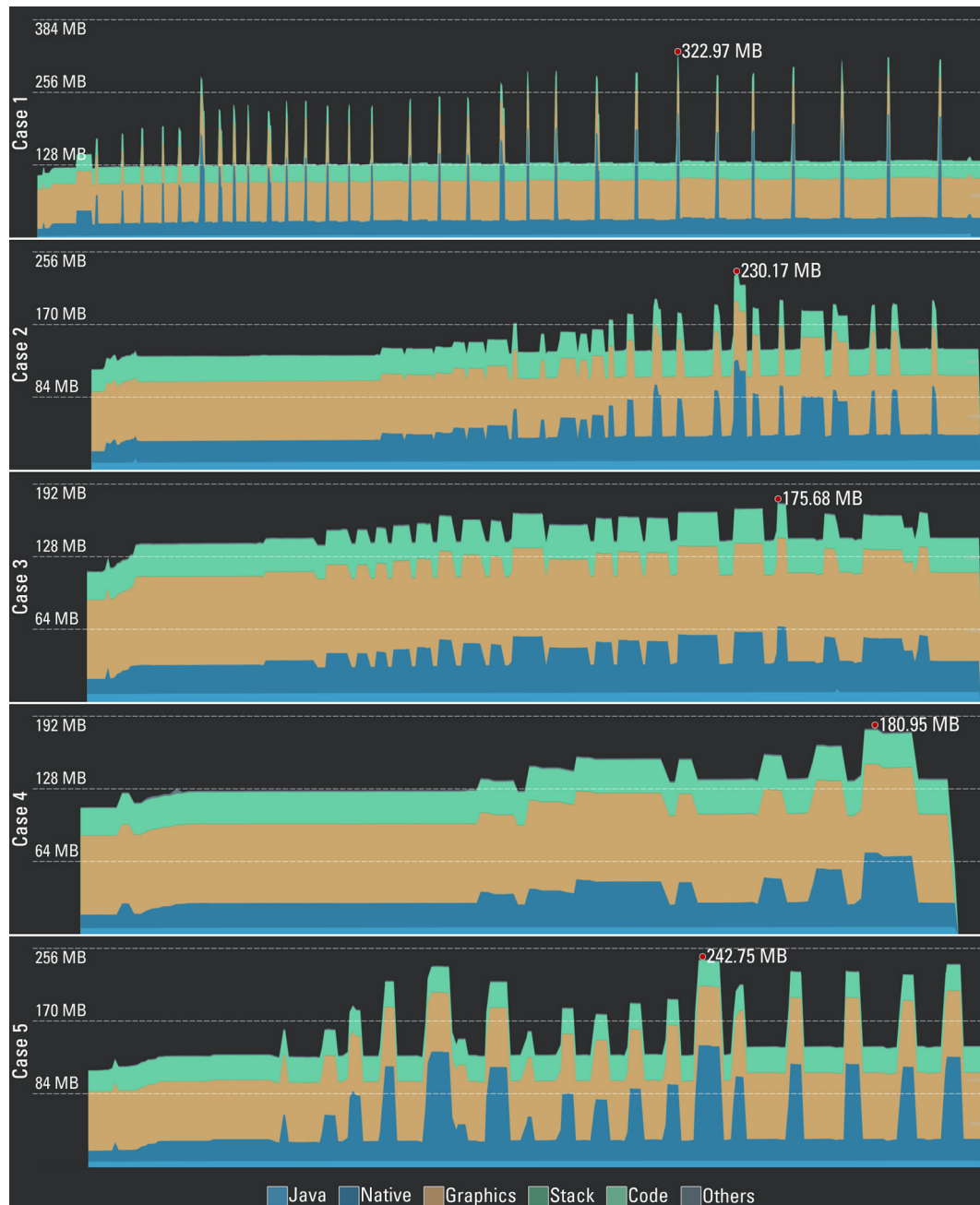
Figure 65 – Memory usage over time of GS-IST running on Galaxy S8. Each test case has a different time scale.
