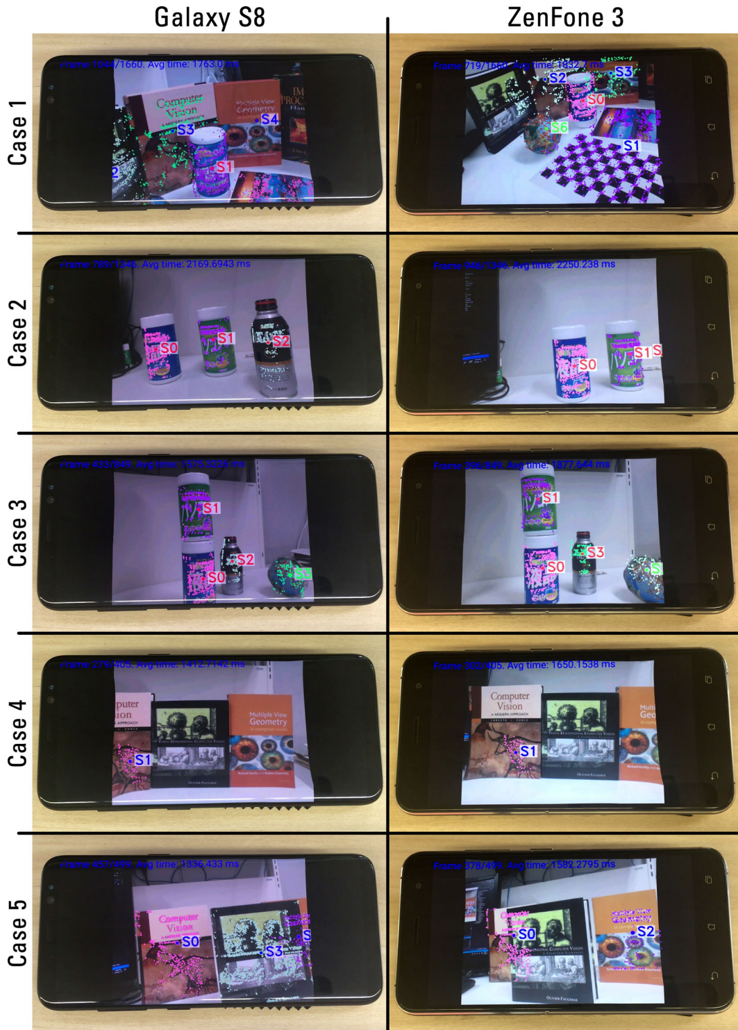
Figure 60 – Results of GS-IST running on a Samsung Galaxy S8 and an ASUS ZenFone 3. Blue labels represent planes, green ones are for spheres and red for cylinders 4 .
