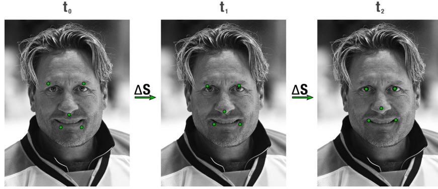
Figure 34 – Cascade shape regressor, in which the landmark position is incremented every stage.
