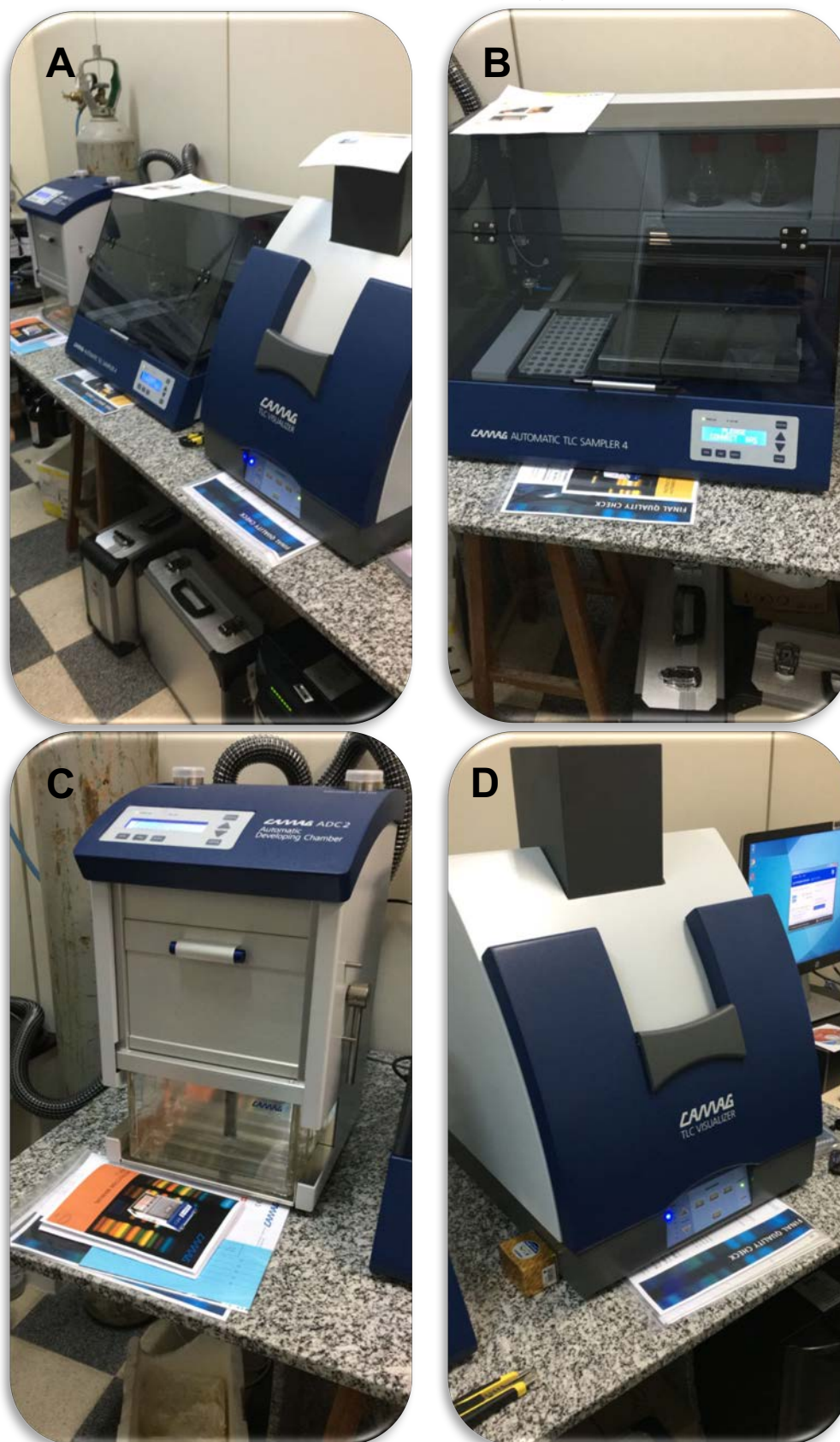
Figura 9 - Módulos CAMAG HPTLC (A); CAMAG Automatic TLC Sampler 4 (B); CAMAG Automatic Development Chamber ADC2 (C); CAMAG TLC Visualizer (D).
