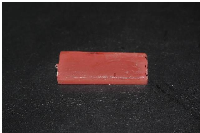
Fig. 10 Amostra de Resina Soft-Comfort (32x10x2,5mm)
