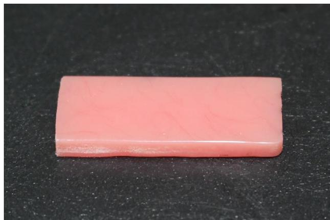
Fig. 07. Amostra de Resina (32x10x2,5mm)
