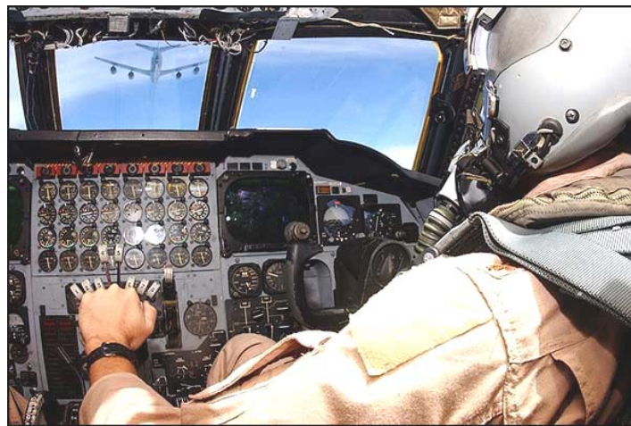
Fig. 4- A complexa interface de controle do Boeing B-52 (foto disponibilizada no site www.marylandaviationmuseum.org/history/b52aircraft.html –15/05/2004)
