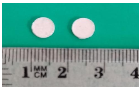
Figure 19 – Image and dimensions of the pellets of BaSO 4 :Eu of this study
