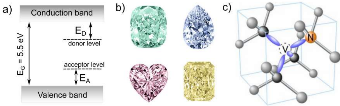
Figure 8 – a) The presence of defects in the diamond host matrix may lead to the creation of donor (acceptor) energy levels (dashed lines) within the wide bandgap of diamond due to the association of electrons (holes) and impurity centers. The energy of the donor, E_D (acceptor, E_A ), and diamond energy gap, E_G are given by solid arrows. b) Colored diamonds containing electronic holes (green), boron (blue), NV color centers (rose) and nitrogen (yellow). c) Schematic representation of the NV defect on a diamond lattice.
