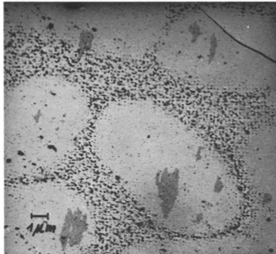
Fig. 2. Same specimen as fig. 1, electron micrograph showing coexistence of the Meissner phase with a phase consisting of flux lines arranged in a square lattice.
