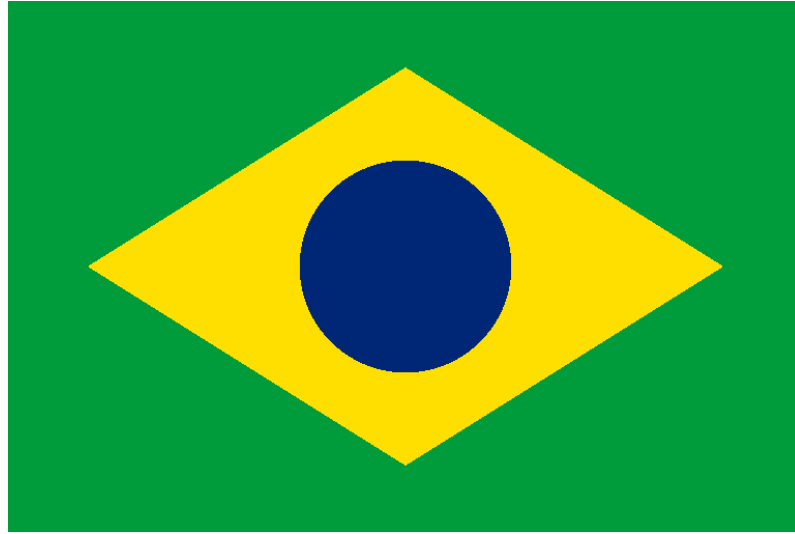
Figure 32 – Permeability field shaped as the Brazilian Flag: Green Rectangle K_1 (Sides: 1.5 \times 1 ), Yellow Diamond: K_2 / K_3 (Diagonals: 1.2 \times 0.75 , check Equation 5.5) and Blue Circle ( R = 0.2 ): Hole.
