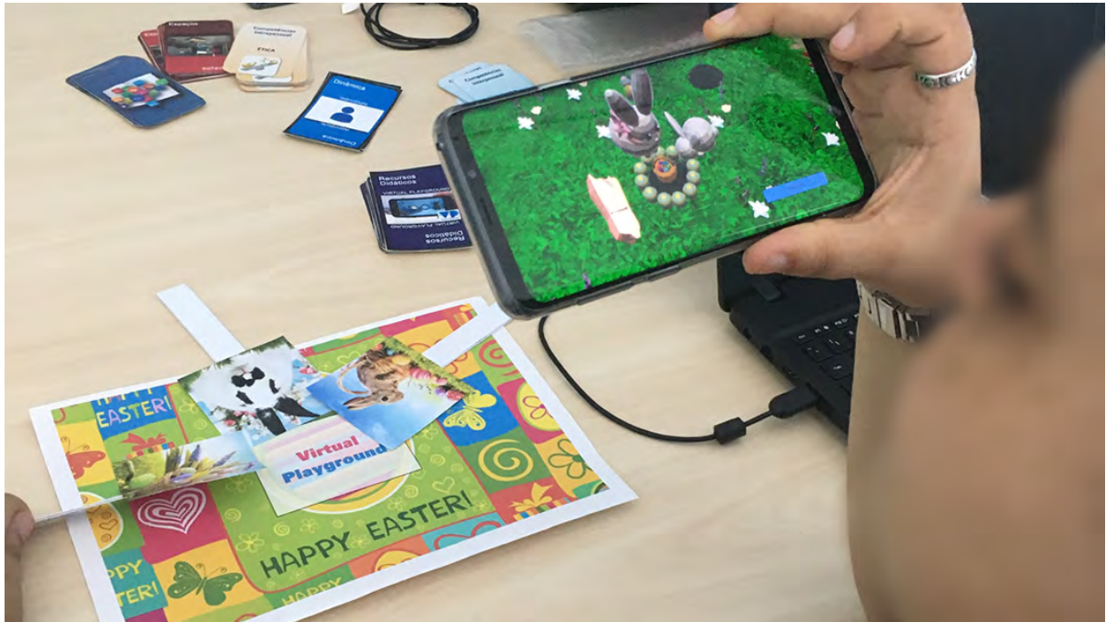
Figure 60 – One of the teachers using Virtual Playground prototype during the second round of testing. The larger paper enables the virtual scenario while each smaller markers with handlers represent a different character the user can move and see it in the mobile phone.
