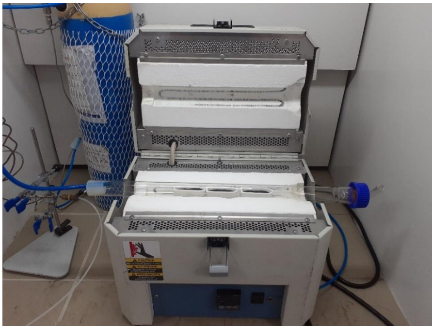
Figura 5 - Reator horizontal tubular com as 3 barquinhas de porcelana contendo as amostras
