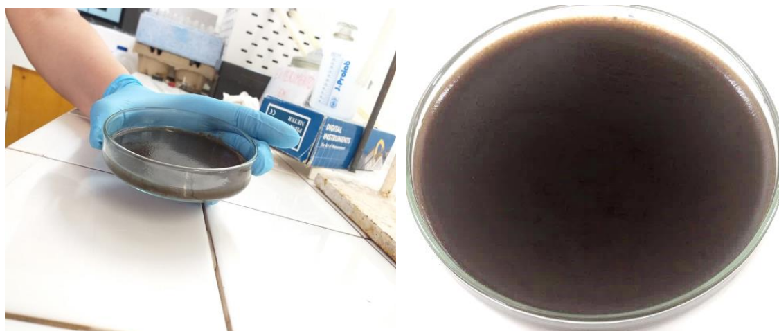
Figure 8 – Photographs of the hydrogel produced with 80% agar and 20% GO
