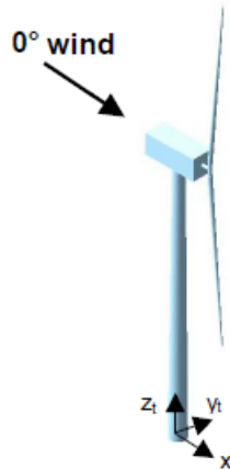
Figure 5 – Tower base wind turbine coordinate system
