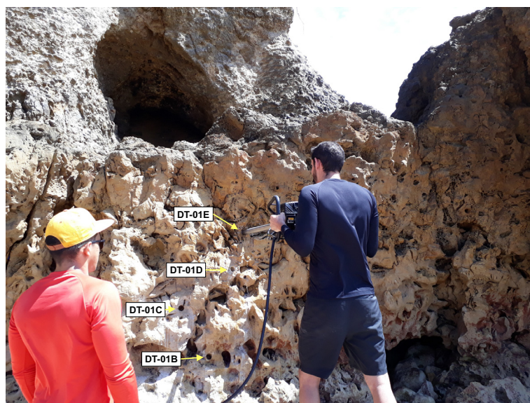
Fig. 4. Example of the samples collected in the field at reef limestone outcrops (DT-01B, DT-01C and DT-01D) of calcarenites of the Tambaba Formation (outcrop DT-01 located in Fig. 1c).
