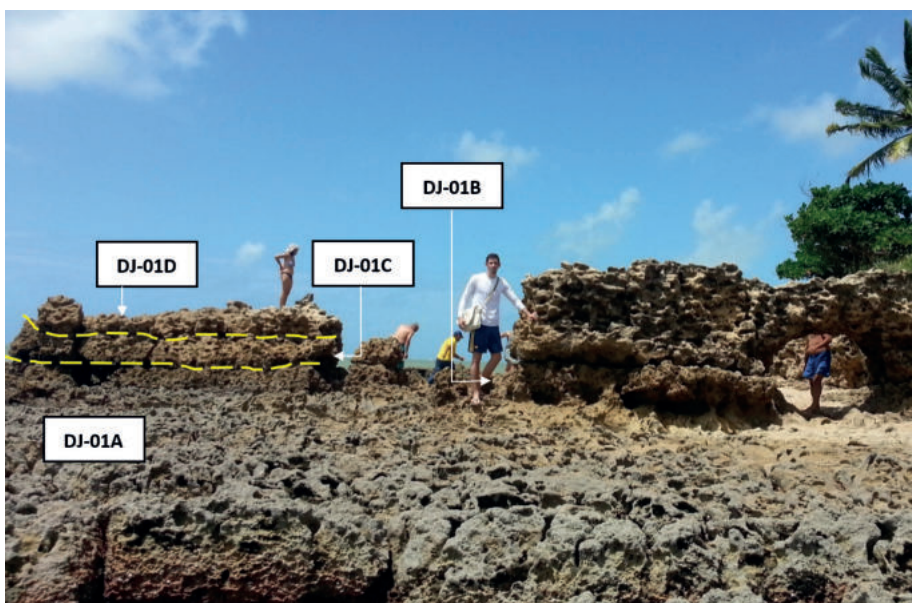
Figure 2 Example of the numbering of the samples collected in the field at reef limestone outcrops (outcrop DJ-01, in Jacumã). The dotted yellow lines show the boundary of the beds.
