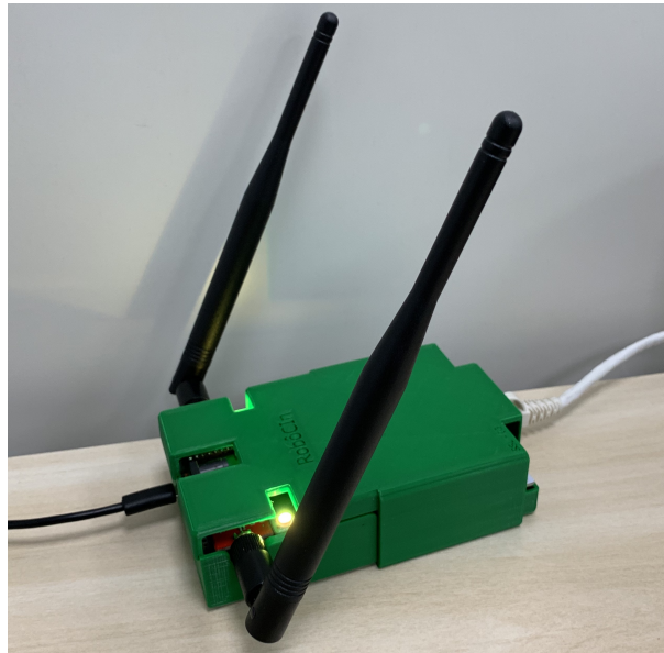
Figure 30 – RobôCIn's base-station, responsible to transmits data from computer to robot, and to receive data from robot to computer.
