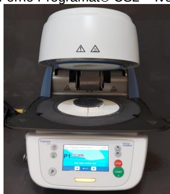
Figura 11 – Forno Programat® CS2 – Ivoclar Vivadent
