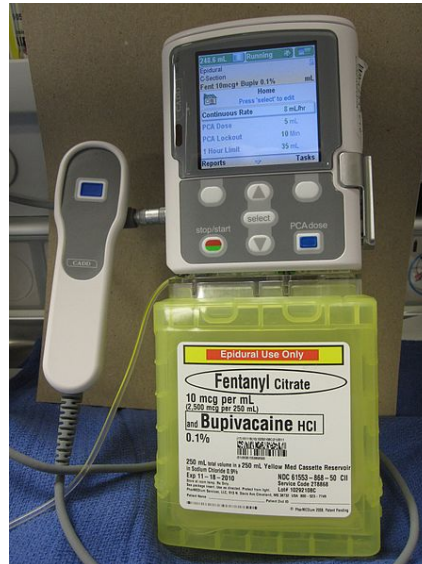
Figure 39 – A patient-controlled analgesia infusion pump.
