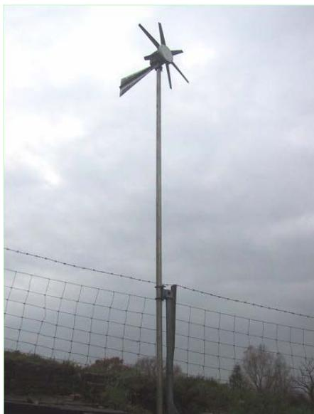
Figura 2.8 – Turbina Eólica Rutland Wincharger WG 910 - Cortesia: MARLEC [15].
