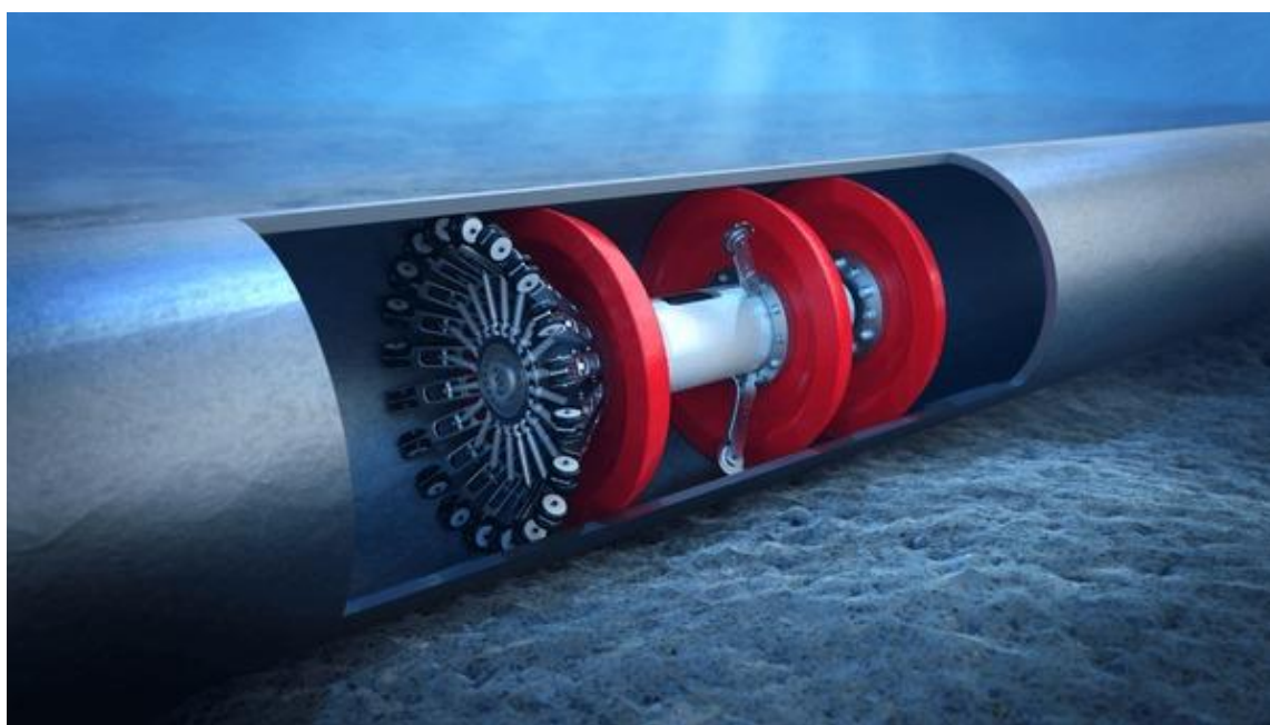
Figura 2 - Pig de In Line Inspection.
