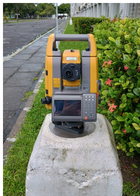
Figure 2. The Topcon GT-605 RTS used in the measurements, in June 2024.
