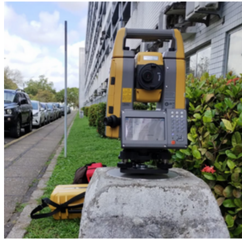
Figure 2. The robotic total station used in the measurements, in February 2024.
