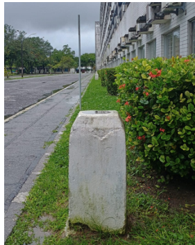
Figure 1. The calibration baseline is composed of seven pillars with forced centering, in June 2024.
