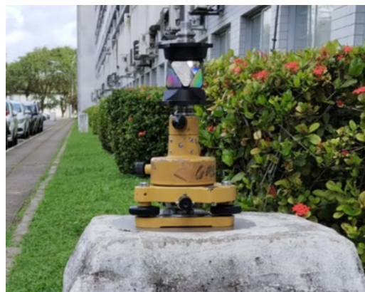
Figure 3. The 360° prism used in the measurements, in February 2024.
