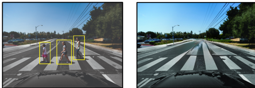
Figure 22 – On the left is the original frame, where the people crossing the street are detected by the ADAS. On the right is the frame received during a replay attack, where the vehicle is misguided to see no one crossing the street.
