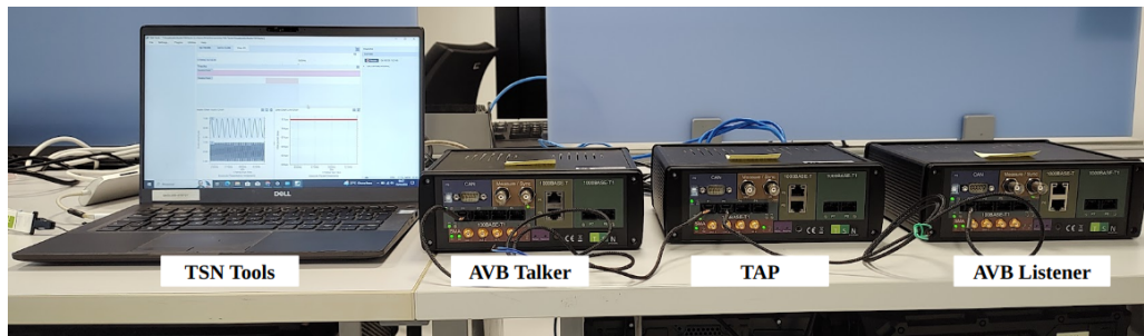
Figure 38 – Automotive-grade devices to simulate an automotive Ethernet network composed of an AVB Talker, a TAP and an AVB Listener to transmit audio signals.
