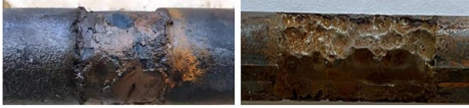
Figure 4.1. Morphology of a corroded subsea pipeline.
