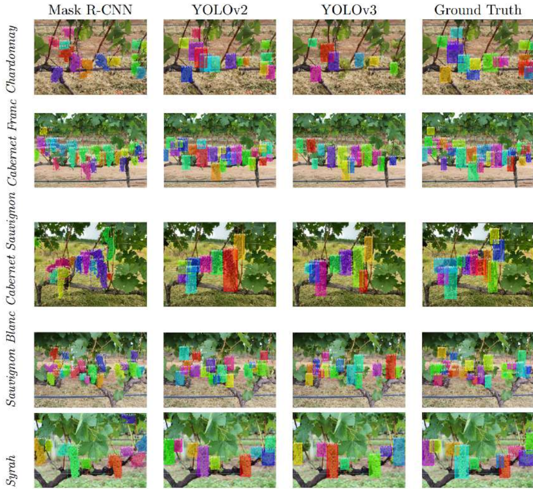
Figure 17 – Object detection results comparison between Mask R-CNN, YOLOv2, and YOLOv3 on grape cluster detection, adapted from (SANTOS et al., 2020). The figure demonstrates the varying performance of each architecture in identifying, localizing, and segmenting grape clusters under real-world vineyard conditions, with Mask R-CNN showing superior precision in cluster localization compared to YOLO variants.
