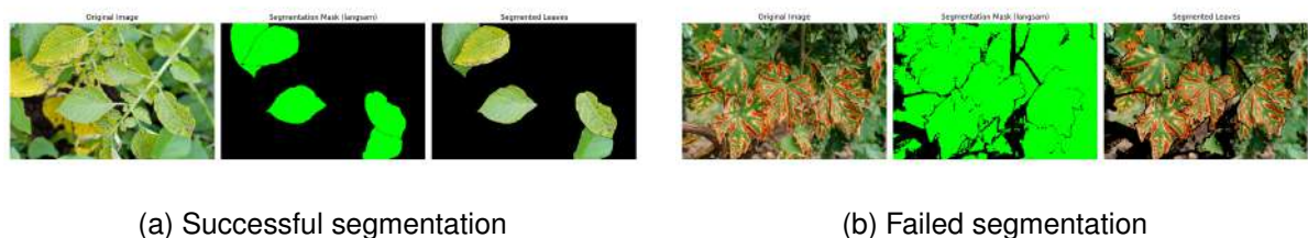
Figure 42 – LangSAM segmentation performance: (a) successful language-guided segmentation using natural language prompts, and (b) limitations in complex scenes where semantic understanding fails.
