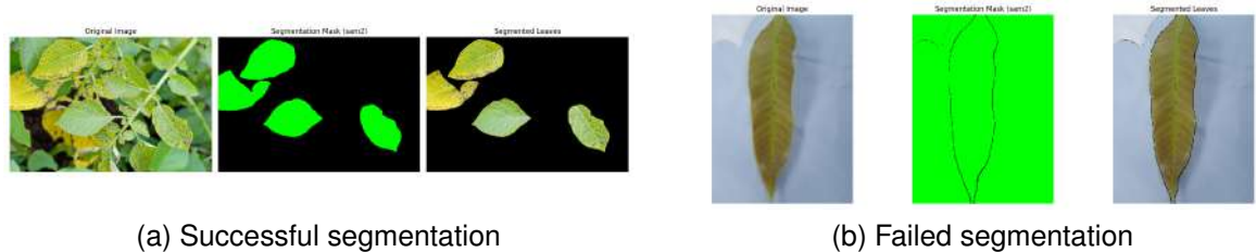
Figure 40 – SAM2 segmentation performance: (a) improved granularity and speed compared to SAM, and (b) challenging scenarios where segmentation quality remains suboptimal.
