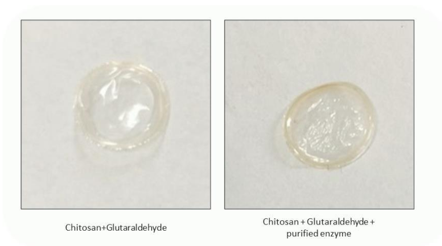
Figure 5. Preparation of Chitosan film. (A) Film in absence of purified enzyme. (B) Film in presence of purified enzyme after immobilization procedure.
