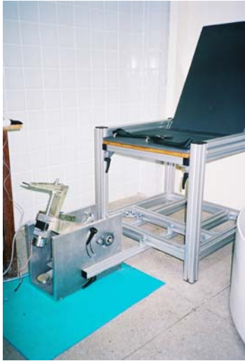
Figure 1 Front view of the transportable ankle ergometer device. The ergometer is composed of the adjustable seat and adjustable footplate box with its electronics.
